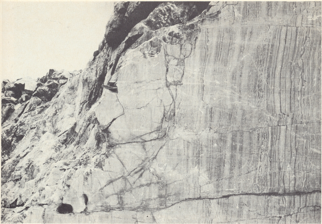
Plate VII.—Irregular joints near surface due to fluctuations in temperature. "Kudu" marble quarry, Karibib 54 (loc. 18). Plaat VII.—Onreëlmatige nate naby oppervlak te wyte aan temperatuurskommeling. "Kudu"-marmergroef, Karibib 54 (lok. 18).
